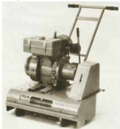
Deck Sealer Under-Carriage showing the No. DS5 Cutter Drum Assembly.
